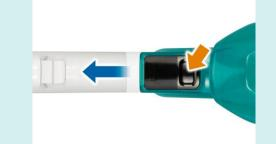
Pipe-lock system secures the pipe to the capsule to prevent it coming out
