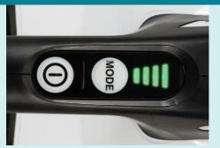
On/off switch, mode selection switch and mode indicator panel
